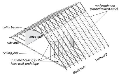
**Finished attic:** This illustration depicts two approaches to insulating a finished attic. Either A) insulate the knee wall and side attic floor, or B) insulate the roof deck.
