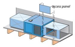
**Plenums, poorly sealed to air handler:** When air handlers are installed in tight spaces, plenums may be poorly fastened and sealed. Cutting a hole in the duct may be the only way to seal this important joint.
