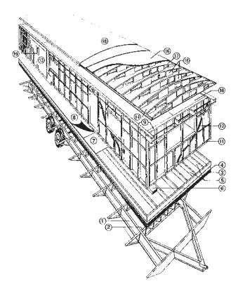
**Typical components of a mobile home:** 1–Steel chassis. 2–Steel outriggers and cross members. 3–Underbelly. 4–Fiberglass insulation. 5–Floor joists. 6–Heating/ air conditioning duct. 7–Decking. 8–Floor covering. 9–Top plate. 10–Interior paneling. 11–Bottom plate. 12–Fiberglass insulation. 13–Metal siding. 14–Ceiling board. 15–BOWSTRING trusses. 16–Fiberglass insulation. 17–Vapor barrier. 18–Galvanized steel one-piece roof. 19–Metal windows.
