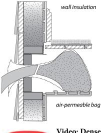
Floor cavities: Floor cavities are difficult to fill in platform-framed homes. Blow a plug of insulation into the floor cavity to insulate this uninsulated area.
