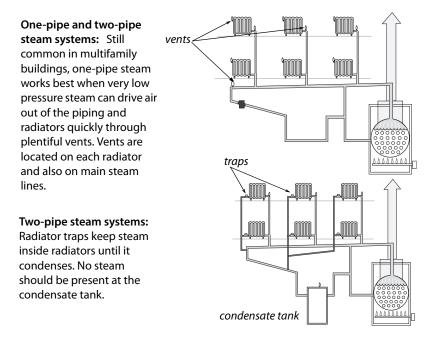
✓ When you can't gain access to all the system's steam traps at the same time, consider abandoning failed steam traps and installing radiator-inlet orifices in two-pipe steam radiators. The orifices limit steam flow to an amount that can condense within the radiator. Orifices can also reduce steam delivery to oversized radiators by 20% or a little more.
