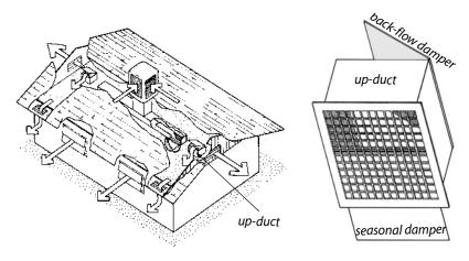
**Air circulation:** Outdoor air is sucked through the evaporative cooler and blown into the home pushing house air out of the partially open windows. Some dwellings with evaporative coolers employ up-ducts instead of open windows for security concerns.
