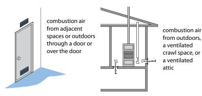
**Combustion air options:** Combustion air can be supplied from adjacent indoor spaces or from outdoors. High vents may occasionally compete with chimney draft for available air. Beware of drawing combustion air from wet crawl spaces. Pick your outdoor combustion-air location carefully to avoid pressurizing or depressurizing the CAZ.
