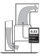
Total external static pressure (TESP): The positive and negative pressures created by the resistance of the supply and return ducts produces TESP. The measurement shown here simply adds the two static pressures without regard for their signs. As TESP increases, airflow decreases. Numbers shown below are for example only.
