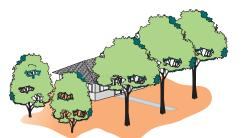
**Roof and window shading:** Tall trees near the south facing walls and broad trees near the east- and west-facing walls are a good shading strategy.
