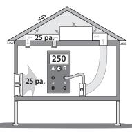
**Measuring duct leakage to outdoors:** Using a blower door to pressurize the house with a duct blower to pressurize the ducts measures leakage to the outdoors a smaller number and a better predictor of energy savings. This test is preferred for evaluating duct leakage for specialists in both building air leakage and duct air leakage.
