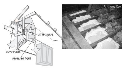
**Kitchen soffits:** The ventilated attic is connected to the soffit and the wall cavity through framing flaws. Any hole in the soffit creates a direct connection between the kitchen and attic. Block off the soffit from the attic with drywall or plywood sealed with two-part spray foam as shown in the photo.
