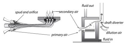
**Natural-draft, open combustion gas burners:** Combustion air comes from the indoors in open combustion appliances. These burners use the heat of the flame to pull combustion air into the burner. Dilution air, entering at the draft diverter, prevents overfire draft from becoming excessive.
