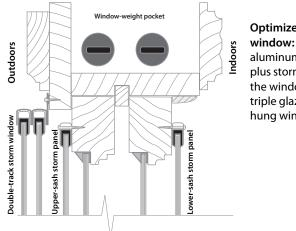
Optimized double-hung window: An exterior aluminum storm window plus storm window panels on the window sashes create triple glazing in this doublehung window.
