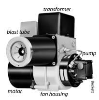
**Oil Burners:** Oil burners are power burners that atomize the oil by pumping it through a nozzle. A blower forces combustion air into the oil mist. Electrodes powered by a transformer light the mixture.
