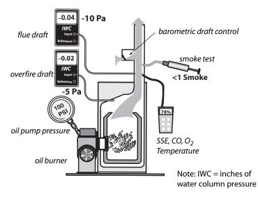
**Measuring oil-burner performance:** Measuring oil-burning performance requires, a manometer, flue-gas analyzer, smoke tester, and pressure gauge.
