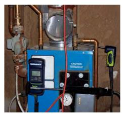
**Combustion analysis:** Measuring  $0_2$  and CO during worst case is an effective way to evaluate the adequacy of combustion air.
