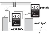
**Measuring draft:** Measure chimney draft *downstream* of the draft diverter.
