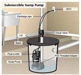
Sump pump: Pumps water out of a sump or basin where water collects in a basement or crawl space.
