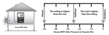
**Building-to-attic pressure:** This test allows the tester to evaluate the attic's two possible air barriers—the ceiling and the roof. The diagram shows how to determine which air barrier is tighter.
