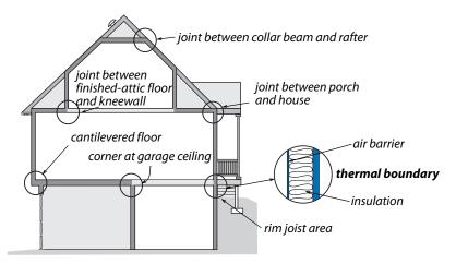
**Air leaks at the thermal boundary:** The air barrier and insulation, which should be adjacent to one another, are located at the thermal boundary. The insulation and the air barrier are often discontinuous at corners and transitions.
