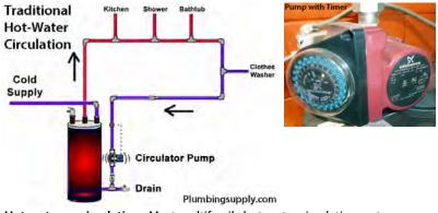
Hot-water re-circulation: Most multifamily hot-water circulation systems return cold water to the water heater and supply hot water to the distribution pipes.
