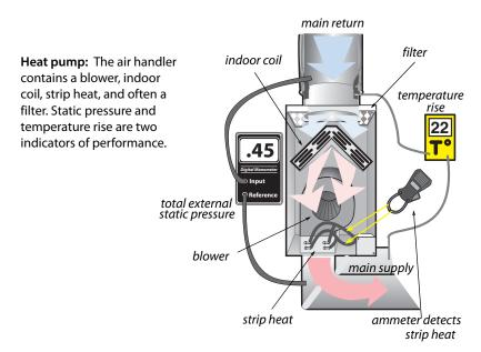
Heat pumps are also equipped with auxiliary electric resistance heat, called strip heat. The energy efficiency of a heat pump depends on how much of the heating load the compressor provides without using the strip heat.
