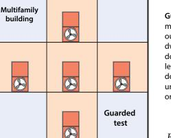
Guarded test: Attempts to measure the leakage to outdoors of a single dwelling unit. One blower door measures the units air leakage while other blower doors pressurize adjacent units to the same negative or positive pressure.
