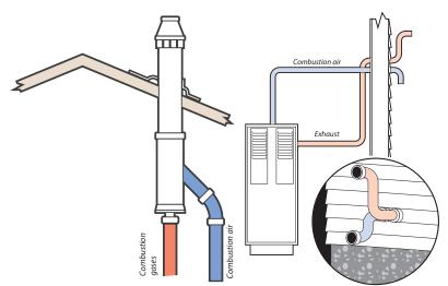
Two types of sealed-combustion vents: On the left is a concentric vent exiting through a roof. On the right is a plastic-pipe vent and combustion-air opens through the wall.
