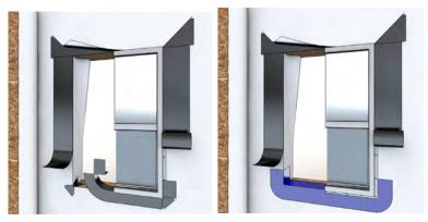
**Flashing nail-fin windows:** Installers place the window on and over the sill flashing. The side and top flashing cover the fastening fin. The two methods shown here are: using a flexible membrane (right) and using a bow-tie-shaped flashing to underlay the corners when using a standard membrane.
