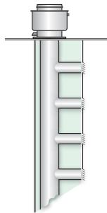
Multifamily exhaust ventilation system: Many multifamily buildings have vertically ducted exhaust ventilation systems with registers opening to kitchens and bathrooms on each floor.
