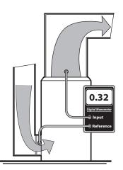
Static pressure and temperature rise: Measure static pressure and temperature rise across the new furnace to verify that the duct system isn't restricted. The correct airflow, specified by the manufacturer, is necessary for high efficiency.
