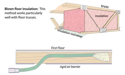
**Blowing floor cavity:** Uninsulated floor cavities can be blown with fiberglass or rock wool insulation, using a fill tube.
