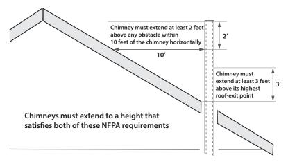
**Chimney terminations:** Should have vent caps and be given adequate clearance height from nearby building parts. These requirements are for both masonry chimneys and manufactured all-fuel chimneys.
