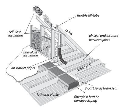
**Finished attic best practices:** Air sealing and insulation combine to dramatically reduce heat transmission and air leakage in homes with finished attics.
