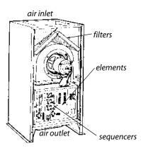
**Electric furnace:** A squirrel-cage blower blows air over 2 to 6 electric resistance coils and down into the plenum below the floor.
