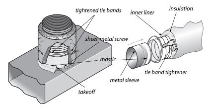
**Flexduct joints:** Flexduct itself is usually fairly airtight, but joints, sealed improperly with tape, can be very leaky. Use methods shown here to make flexduct joints airtight.
