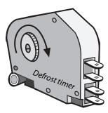
**Defrost Timer:** The defrost timer initiates the defrost cycle to melt ice at regular intervals.
