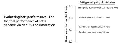
Installers must cut and fit batts very carefully. Batts achieve their advertised R-value only when they are touching all six sides of the cavity it inhabits.
