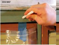
First, crush the capsule and shake it to mix ingredients. Then swab the sample for 30 seconds.
