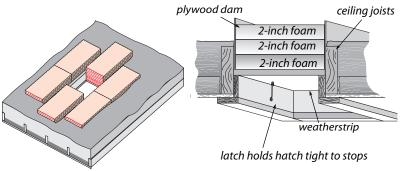
**Batts form attic-insulation dam:** Where head space is limited, fiberglass batts are a good choice for a low-profile insulation dam. **Insulated attic hatch:** Building a dam prevents loose-fill insulation from falling down the hatchway. Foam insulation prevents the access hatch from being a thermal weakness. Install foam to achieve attic-insulation R-value of R-38. Foam can be glued together in layers.
