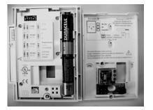
Many models of programmable thermostats have settings that you select from inside the thermostat. These settings include the heat-anticipator setting, which adjusts the cycle length of the heating or cooling system.
