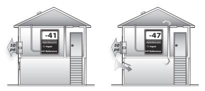
**Zone connectedness:** The attic measures closer to outdoors after the basement window is opened, indicating that the attic and basement are connected by a large bypass.
