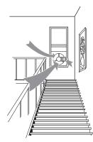
Window fans: Window fans circulate outdoor air when it is cooler than indoor air. The air circulation removes heat from the house.
