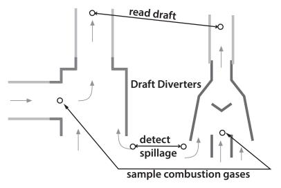
**Testing locations:** This illustration shows two draft diverters and the locations (circles) for draft testing, spillage detection, and sampling of combustion gases.
