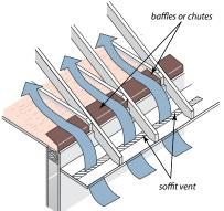
Ventilation pathways: Install baffles or chutes in every roof bay where soffit or eave venting exists.
