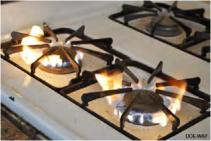
Flame observation: Unstable flames with yellow tips indicate poor combustion and possible CO production.
