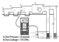
Total duct air leakage measured by the duct blower: All registers are sealed except the one connecting the duct blower to the system. Pressurize the ducts to 25 pascals and measure airflow.
