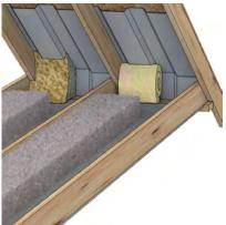
**Insulation at the eaves:** Stuff fibrous insulation or spray foam into the eave area to maximize R-value. Use mechanical fasteners to attach the baffles to the framing.
