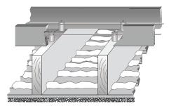
Shielding knob and tube: If you can't decommission knob-andtube wiring, you may construct a dam to shield the wiring from insulation.
