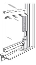
**Lifting an upper window sash:** First cut paint away from around the sash inside and outside. Then lift with leverage or a jack.
