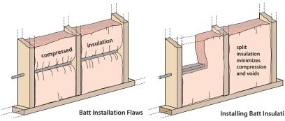
**Fiberglass batts, compressed by a cable:** This reduces the wall's R-value by creating a void between the insulation and interior wallboard. **Batt, split around a cable:** The batt attains its rated R-value.
