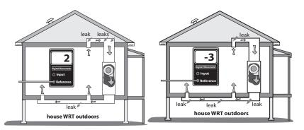
**Dominant return leaks:** When return leaks are larger than supply leaks, the house shows a positive pressure with reference to the outdoors.
