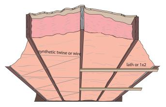
**Floor insulating with batts:** Use unfaced fiberglass batts, installed flush to the floor bottom, to insulate floors. The batt should fill the whole cavity if it is supported by lath or plastic twine underneath.
