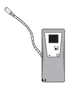
**Gas sniffer:** Use this device to detect the presence of combustible gases around fittings.
