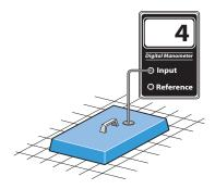
If the ducts are in a basement and the basement is conditioned, pressure pan testing isn't necessary, although air sealing the return ducts for safety is still important.
