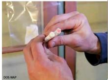
Red means lead-positive and white means lead-negative.
