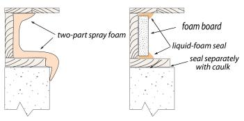
**Foam-insulated rim joists:** Installing foam insulation is the best way to insulate and air seal the rim joist.
