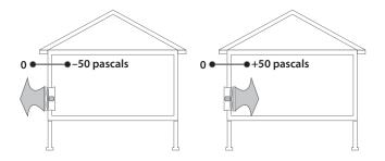
Conducting the Blower-Door Test
