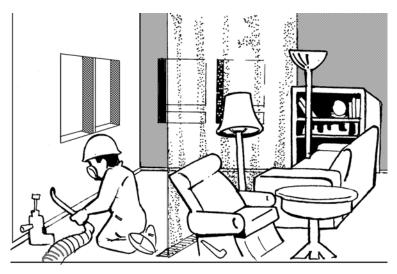
**Protective sheeting:** Dust-tight floor-to-ceiling barriers must separate work areas from living areas, according to EPA's RRP rule.
