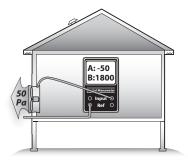
**Blower-door test:** Air barriers are tested during a blower-door test, with the house at a pressure of 50 pascals negative with reference to outdoors. This house has 1800 CFM<sub>50</sub> of air leakage. Further diagnostic tests can help determine where that leakage is coming from.
