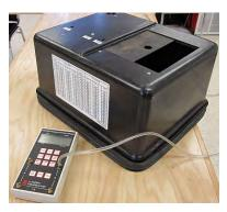
**Measuring fan airflow:** Use an exhaust-fan flow meter or a flow hood to verify the airflows through local exhaust fans and whole-building ventilation fans.
