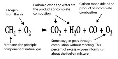
Modern combustion analyzers measure  $O_2$ , CO, and flue-gas temperature. Some models also measure draft. Combustion analyzers also calculate combustion efficiency or steady-state efficiency (SSE), which are synonymous.
