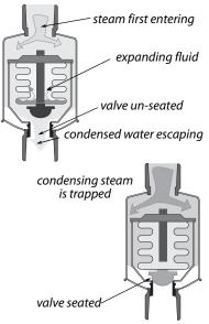
**Steam traps:** Steam enters the steam trap heating its element and expanding the fluid inside. The expanded element plugs the steam's escape with a valve.
