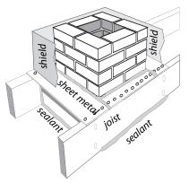
**Sealing around chimneys:** Chimneys require both an air seal and a shield if retrofit insulation is installed with air sealing.
