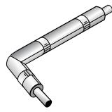
**Properly installed pipe insulation:** Must be the right size for the pipe, must completely cover the pipe, including bends, and must be fastened tightly to the pipe.
