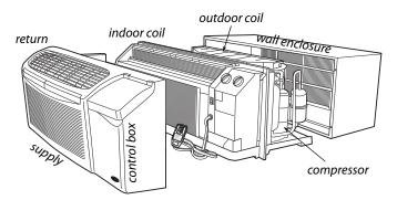
Unitary heat pumps: These unitary ductless heat pumps sit inside an exterior wall. They are a very efficient kind of electric heating and cooling.
