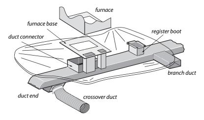
**Mobile-home ducts:** Mobile-home ducts leak at their ends and joints — especially at the joints beneath the furnace. The furnace base attaches the furnace to the duct connector. Leaks occur where the duct connector meets the main duct and where it meets the furnace. Branch ducts are rare, but easy to find, because their supply register isn't in line with the others. Crossover ducts are found only in double-wide and triple-wide homes.
