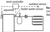
**Reset controller:** This control adjusts circulating-water temperature depending on the outdoor temperature.
