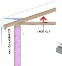
Ice damming: When a roof is unventilated, the home's heat loss warms the roof deck melting snow. The water re-freezes at the eaves and causes moisture damage. **Rooftop foam insulation:** The IRC code requires foam insulation over the structural sheathing when the roof is unventilated.
