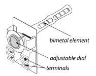
Fan/limit control: Turns the furnace blower on and off, according to temperature. Also turns the burner off if the heat exchanger gets too hot.
