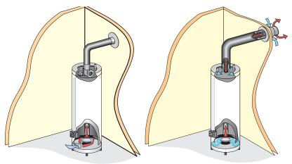
Fan-assisted water heater: The fan allows horizontal venting. The water heater may be open combustion or sealed combustion. **Direct-vent water heater:** Moves combustion air and flue gases through a concentric pipe system without a draft fan.
