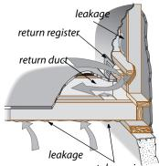
metal panning Panned floor joists: These return ducts are often very leaky and may require removing the panning to seal the cavity.
