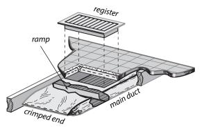
Sealing the end of the main duct: The main duct is usually capped or crimped loosely at each end, creating a major air leakage point. Seal this area and improve airflow by installing a sheet metal ramp, accessed through the last register, inside the duct. Seal the ramp to the ductwork with metal tape and silicone or mastic.
