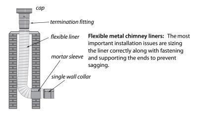
Flexible liners require careful installation to avoid a low spot at the bottom, where the liner turns a right angle to pass through the wall of the chimney. Comply with the manufacturer's instructions, which usually require stretching the liner and fastening it securely at both ends, to prevent the liner from sagging and creating a low spot.
