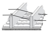
Knob-and-tube wiring: Replace obsolete and worn wiring during energy retrofit work so that workers can insulate building cavities sufficiently.
