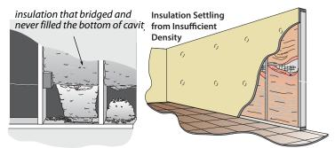
**Problems with low density insulation:** Blowing insulation through one or two small holes usually creates voids inside the wall cavity. This is because insulation won't reliably blow at an adequate density more than about one foot from the nozzle. Use tube-filling methods whenever possible, using a 1.5-inch hose inserted through a 2-inch or larger hole.
