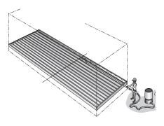
Blowing crosswise cavities: Blowing insulation into belly is easy if the floor joists run crosswise. However, the dropped belly requires more insulation than a home with lengthwise joists. Blowing lengthwise cavities: Floors with lengthwise joists can rarely be filled completely from the ends because of the long tubing needed. The middle can be filled from underneath.
