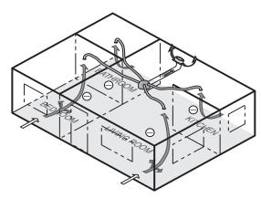
Multi-port exhaust ventilation: A multi-port ventilator creates better fresh-air distribution than a single central exhaust fan.
